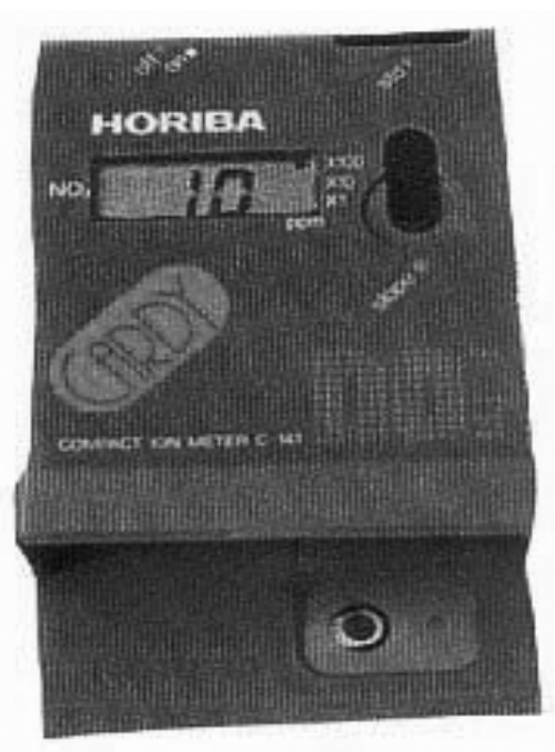
Figure 13.1 Horiba specific ion electrode meter. There are three different meters, one for determining nitrate ( \text{NO}_3 ), one for potassium (K), and another for calcium (Ca). The K- and Ca-specific ion meters require some sample manipulation to ensure that reliable analytical results are obtained.
